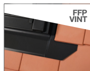
PLAIN TILE For installation into plain tiles, max. overlapped thickness is 28 mm (2x14 mm), max. length is 340 mm. Suitable for a roof pitch range of 25° - 90°.
